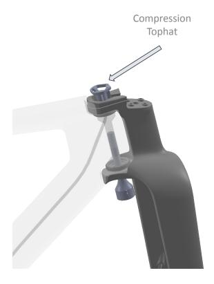
Apply dielectric grease to the outside of all alloy components contacting carbon, hand thread the compression rod to the upper bearing centering compression tophat.
