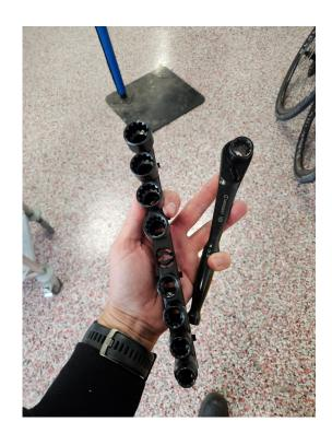
A high quality 14mm pass-through socket is strongly recommended for tightening the collet.
