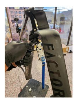
Place the end of a 14mm or passthrough ratchet on the 14mm Collet land. Pass a 6mm allen key through this wrench or socket. Hold the tension rod static with the 6mm Allen while turning and tightening the 14mm ratchet. Tighten to a max of 8Nm, or until snug. Caution must be taken here to not spin the preload rod HS will become over tight.
