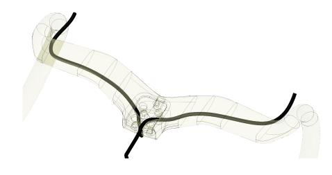
Snake hoses the hoses coming from the top of the frame and fork through the bar, respecting which is left and which is right and corresponding front/rear brakes
