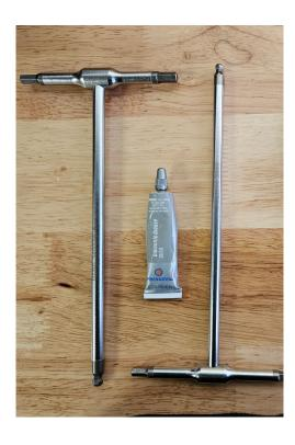
High quality T-Handle hex wrenches (6 and 5mm) are recommended for the next steps. A high quality dielectric grease acts to insulate the aluminium compression rod from the carbon and prevent galvanic corrosion from occurring. Many conventional greases also have dielectric (non-conductive) properties.
