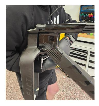
Place the end of a 14mm or passthrough ratchet on the 14mm Collet land. Pass a 6mm allen key through this wrench or socket. Hold the tension rod static with the 6mm Allen while turning and tightening the 14mm ratchet. Tighten to a max of 8Nm, or until snug. Caution must be taken here to not spin the preload rod HS will become over tight. You may find it helpful to brace your arm against the fork to hold the preload rod static.
