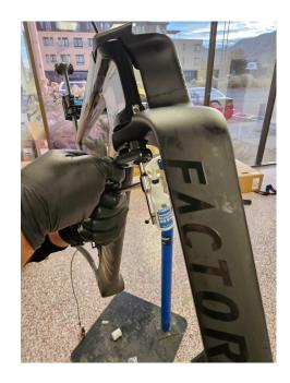
Insert and tighten the setscrew into the underside of the tension rod/collet assembly to lock the collet in place. Ensure the Loc-Tite blue is in place, and add a dab if reinstalling.
