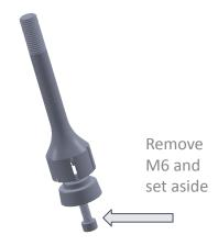
Prep the tension rod by ensuring interface with the collet is well greased. Thread the collet in until it lightly contacts the tension rod. Lightly grease the M6 bolt but don't install yet. Verify the rotation stop is installed.
