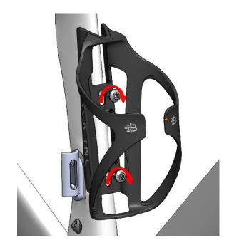
Install cages of your choice and tighten M5 bolts with a high quality 3mm Hex head to **2 Nm.**
