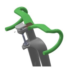
Incline the handlebar to the left or the right, and install the compression cover to no more than 1.5Nm
